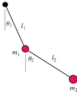
FIG. 1: (Taken from Wolfram Scienceworld) A schematic diagram of the double pendulum, consisting of two masses  $m_1$  and  $m_2$ , connected to massless rods. The dynamical variables that we will model are  $\theta_1$  and  $\theta_2$ , defined in the figure.
